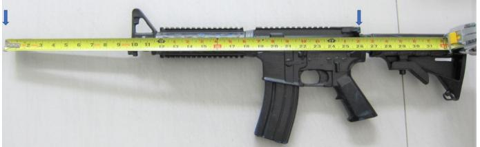
Per the example above, position the lower leg so that the distance from the inside of the muzzle cup to the center of the charging handle slot is 26". You may need to trim the length of the lower leg slightly if you are using a shorter barrel length.
