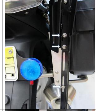
The shield attaches to the lower leg with two M5 x 12 Torx bolts. If you need to remove the lower leg, **mark the depth relative to the main mount** so that you can reassemble it correctly. Position the shield so that it deflects the main exhaust flow. If necessary, extend the shield down slightly past the end of the lower leg.
